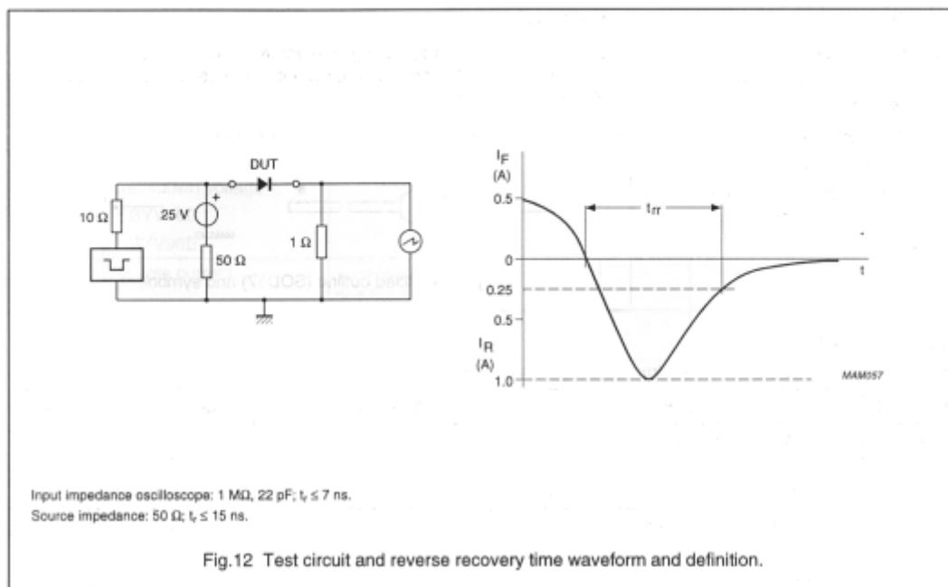
Fig.12 Test circuit and reverse recovery time waveform and definition.
