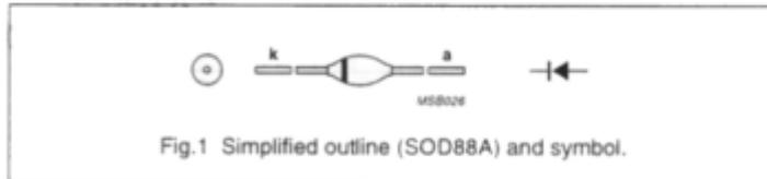
Fig.1 Simplified outline (SOD88A) and symbol.
