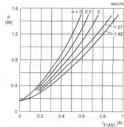
$a = I_{F(\text{RMS})}/I_{F(\text{AV})}$ ;  $V_R = V_{RW\text{Max}}$ ;  $\delta = 0.5$ .
